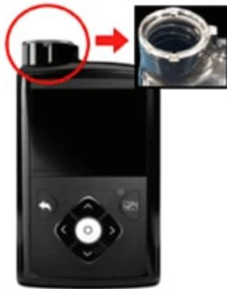
Image: Location of the retainer ring on the MiniMed™ 600 series insulin pump
