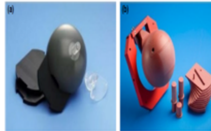
FIG. 4. (a) Elekta ABS and (b) Elekta Solid Water spherical phantoms (reprinted with permission from Elekta Instrument AB). The ABS phantom has a slot to accommodate different inserts (shown in figure) that hold an ionization chamber, cut film, or TLDs. The Solid Water phantom has plug-like inserts (shown in figure), which must be drilled to accommodate the ionization chamber. A single film or a stack of films can also be irradiated inside this phantom using the inserts shown. The ABS phantom attaches to the Perfexion/Icon PPS (i.e., the treatment couch) using the special phantom holder shown in Fig. 1, whereas the Solid Water phantom attaches to the PPS using the patient frame adapter. [Color figure can be viewed at wileyonlinelibrary.com ]
