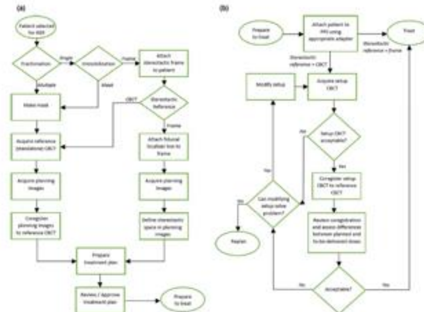
FIG. 13. (a) Flowchart describing steps leading up to patient treatment with Elekta GSI devices. (b) Flowchart describing treatment setup steps for Leksell Gamma Knife device. [Color figure can be viewed at wileyonlinelibrary.com ]
