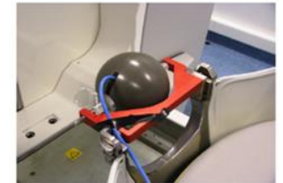
FIG. 1. Illustration of the ionization chamber orientation that was used for the Elekta Monte Carlo simulations to determine the k_{Q,clin} factor in the Elekta ABS phantom. The red phantom holder, which attaches to the patient couch and holds the ABS phantom, is also included in the Monte Carlo simulations. (Reprinted with permission from Elekta Instrument AB.) [Color figure can be viewed at wileyonlinelibrary.com ]
