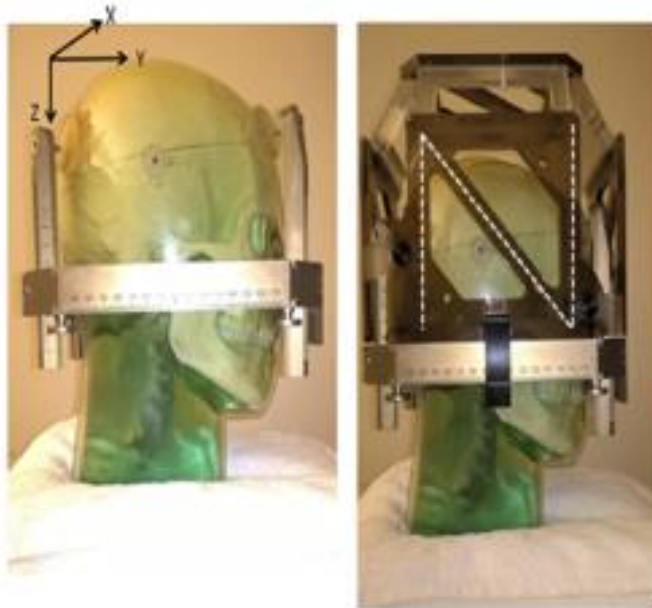
FIG. 12. Leksell headframe on phantom (left) and with MR indicator box (right). The fiducial channels, which are filled with copper sulfate, are outlined by dashed lines. The origin of the Leksell coordinate system is at the superior-right-posterior corner of the fiducial box, and the positive directions of the x, y, and z axes are as shown in the figure. [Color figure can be viewed at wileyonlinelibrary.com ]
