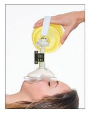
EMMA can be used with a breathing circuit to provide CO2 measurements
